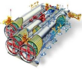
Fig. 9.10 Hydrostatic vertical continuous bottle sterilzer.
